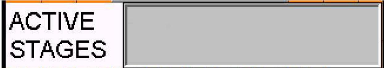
Displayed at the top of the screen is the Active Stages indicator. This text field will display what heat/cool stage is currently active. In instances where no stage is active the text field will display "None". The text field will also indicate if an error has occurred and the system is put into shutdown.
