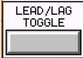
Under pump controls you'll find the Lead/Lag toggle button. This is a standard pushbutton. Pressing it will change the lead pump to lag and lag pump to lead. This effectively switches which pump is on for the remainder of the lead/lag 7-day schedule
