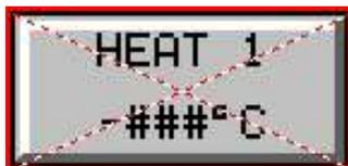
Once access has been granted to the change set point screen, you can edit the water heat and cool set points. The set points are buttons and have some fading around the parameter, indicating that they are editable. To edit these set points, press the set point button. A number pad pops up, enter the appropriate set point and press enter.
