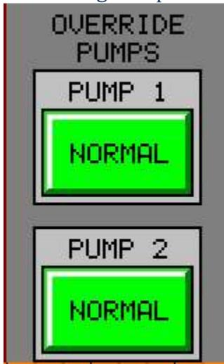
Indication that the pumps are working come from a flow switch. The flow switch closes when water is flowing in the system from a pump. It is possible for the flow switch to get damaged or malfunction. The program determines that the pumps aren't working if it doesn't receive this feedback from the flow switch. The Override feature should be utilized under these circumstances to force a pump to run.
