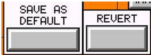
Once new set points have been entered they can be saved by pressing the “Save As Default” button at the bottom of the screen. If a set point is changed accidentally, pressing the “Revert” button will change all staging set points back to what is saved as default. The set points will also revert back to what is saved in the case of a system reboot. This Save and Revert system can be found on the Alarm Set point screen as well, more below.
