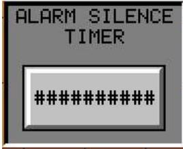
The Silence button appears whenever an Alarm is present. The amount of time the alarm can be silenced is configurable from this Set Point Edit screen. The timer is read in seconds, so an allowed silence time of 1 hour would require the operator to enter the number 3600. Being that there are 3600 seconds in an hour.
