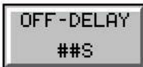
The OFF-Delay is similar to the ON-Delay except this is the amount of time the stage will stay energized after the stage set point has been satisfied.
