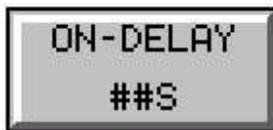
Both Heating and Cooling have an ON-Delay timer that counts down before a stage is initiated. The default for these timers is 4 seconds. Ex. If the Cool 1 stage set point is 100 degrees F the loop temperature must be over that cool set point temperature for 4 seconds before the Cool Stage 1 will energize.
