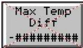
Alarms will be displayed in an Alarm Text Field that appears when a trouble is found. All protective measures will be returned as normal once the corresponding alarm has cleared.
