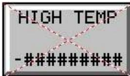
If the return water rises above the High Temp set point the High Temp Alarm will sound. This alarm will disable the Heat Stages of the system.
